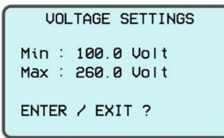
Single phase minimum and maximum operating voltage value is written in the menu that opens. To adjust, press the "SELECTION BUTTON" and enter the value into the box selected with the "UP" and "DOWN" buttons.
