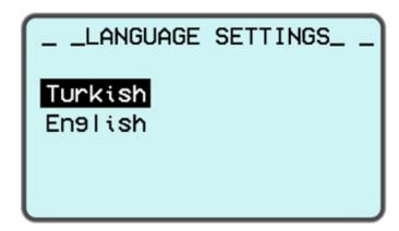
Press the **"UP"** and **"DOWN"** buttons on the screen that opens, highlight the desired language and press the **"SELECTION BUTTON"**.
