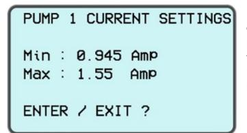
In the menu that opens, minimum and maximum operating current values are written. To adjust, press the **"SELECTION BUTTON"** and enter the value into the box selected with the **"UP"** and **"DOWN"** buttons. NOTE: Writing 10% more and lower motor tag value is ideal for pump protection.
