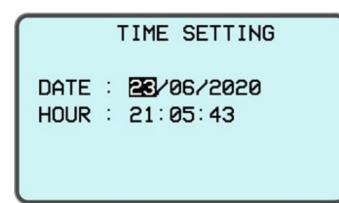
By pressing the "**UP BUTTON**" on the screen that opens, the value in the selected box is increased. After entering the desired value, it waits for 2 seconds and the box automatically moves to the right. Confirmation is done automatically after all settings are made. Date settings are made as day / month / year, time settings are made as hour / minute / second.
