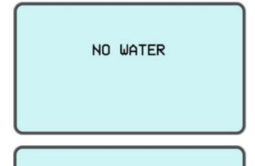
No water error means that the water in the tank is running out and stops the system from working. In the event of an error, the tank is checked and if there is still water in the tank, contact the authorized service.
