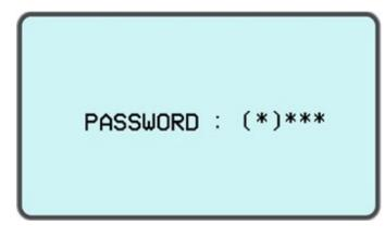
When the correct password is entered, the service settings page opens. Incorrect password entry leads to the previous menu. Press "BACK BUTTON" to exit without entering password.
