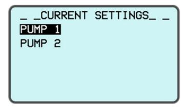
Current value must be entered for each pump in the menu that opens. For the selection of the related pump, scroll with the "**UP**" and "**DOWN**" buttons and press the "**SELECTION BUTTON**".
