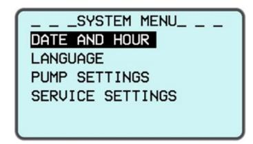
Press the "**MENU BUTTON**" once to access the system menu. Press the "**UP**" and "**DOWN**" buttons on the menu to enter, and press the "**SELECTION BUTTON**".
